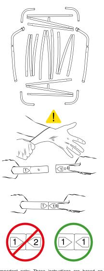
Important note: These instructions are based on assembling the 3m version. Other size kits will have slightly different configurations of poles but can still be assembled in the same way.
